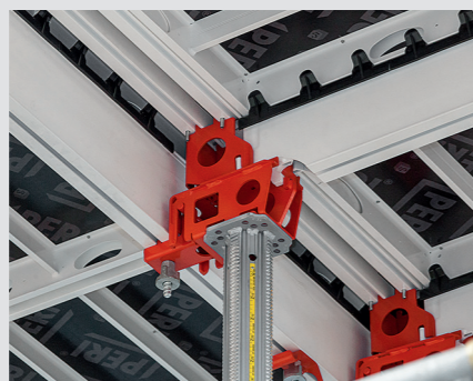
The directional change provided by the drophead allows the direction of the main beam to be changed in the standard system.
