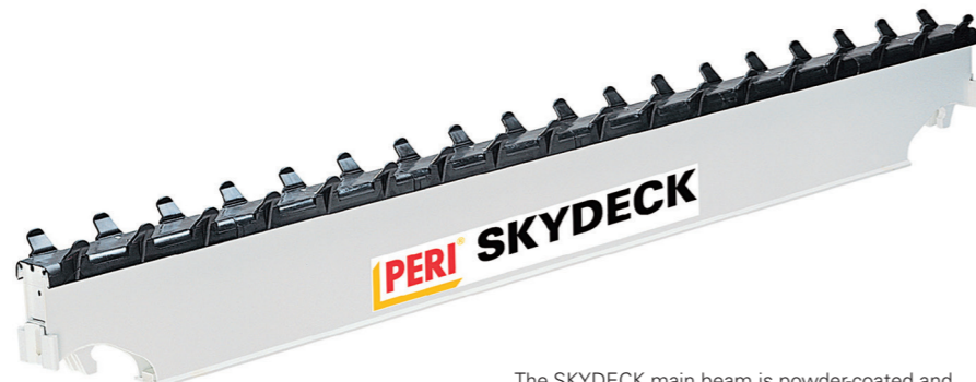
The SKYDECK main beam is powder-coated and the rack is made of plastic. This prevents adhesion of the concrete and minimizes cleaning requirements.
